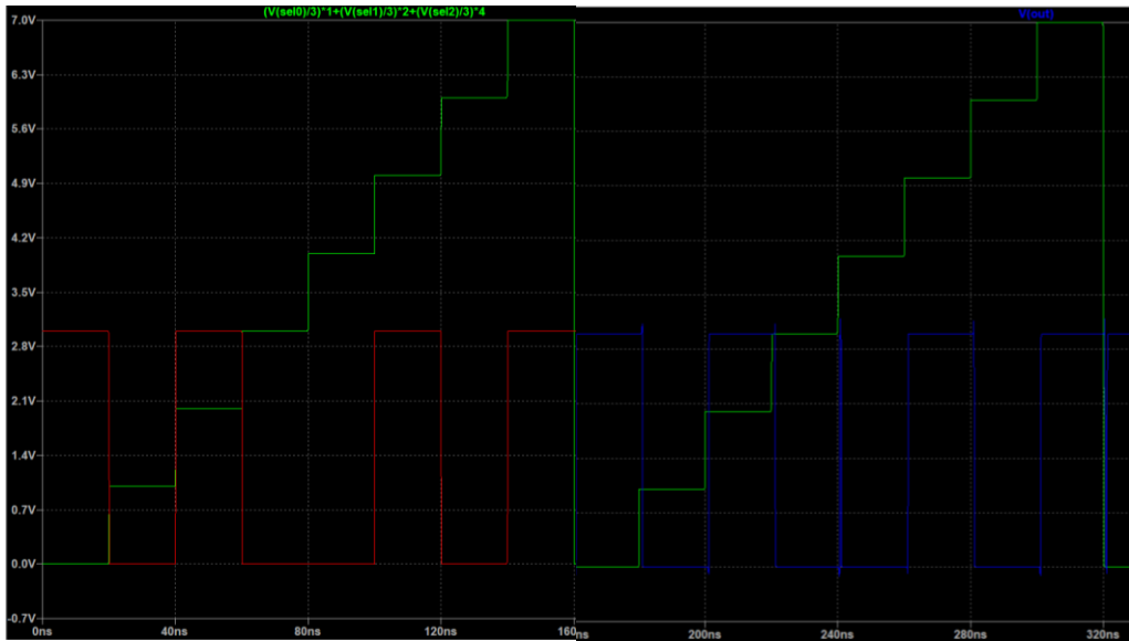
Figure 7: LTspice waveform of register file test
